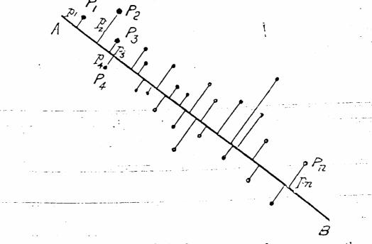
Now clearly  $U=S(p^2)$  is the moment of momentum, the second moment of the system of points, supposed equally loaded, about the line AB. But the second moment of a system about a series of parallel lines is always least for the
